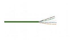
Kramer's BCLS-21 is a high-performance CAT 6 U/UTP cable designed for IT, LAN and Ethernet installations. It is constructed with four pairs of 23AWG solid bare copper conductors with a cross filler. It is enclosed in an LSZH jacket with internal rip cord and sequential markings every meter and packed in a Reelex II carton for easy to pull-out. BCLS-21 cable exceeds CAT 6 specifications to provide additional performance and bandwidth beyond the basic standard
